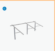
Install the Pre-assemble Support. Fasten the rail with C Clamp Kit on the Post Plate & U post
