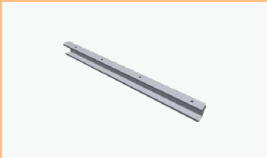
Side Beam Hoop Spec : C10*50*15*2*L2800 Material : Q235B(Hot-Dip Galvanized)
