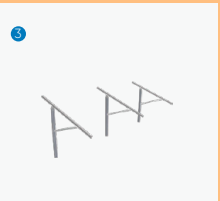
Install the Pre-assemble Support. Fasten the rail with C Clamp Kit on the Post Plate & U post
