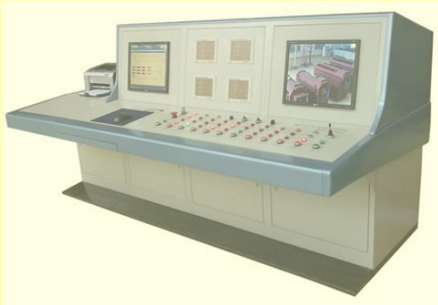
Comprehensive experimental platform for power transformer
