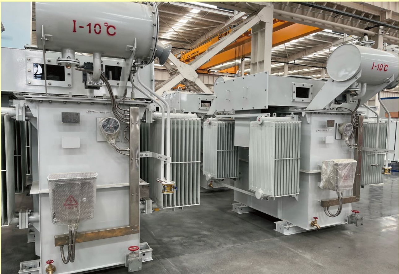
33kv-3150kva Oil immersed transformer
